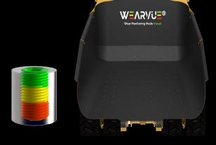
Above housed screw indicator has been installed into the high wearing areas of the truck body
